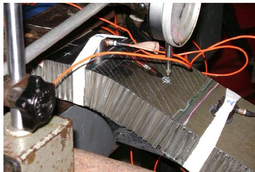
Fig.4. Buckling failure and deformed configuration of the sandwich beam
